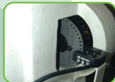
Simple and reliable pulse-counting mechanism is installed for mold height adjustment.
