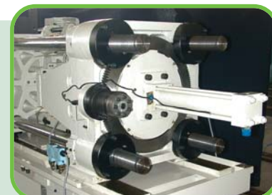
Precise gear type mold height adjustment system.
