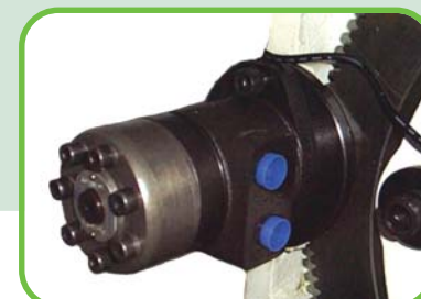
Hydraulic motor powers the Mold Height Adjustment System.
