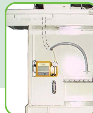
Automatic lubrication maintains a stable, non-wearing condition for longer toggle service life. Lub oil is re-circulated to minimize oil wastage.
